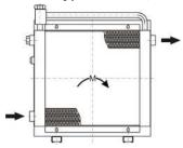
The oil inlet and outlet is always on the same side of the cooling The oil inlet is always at the bottom left of the cooling battery. The second connection must be closed. The oil outlet is always on the opposite side.
