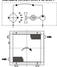
The oil inlet is on the left of the cooling battery. The oil outlet is The oil inlet is on the bottom left of the cooling battery. The second connection at the top must be closed. The oil outlet is always on the opposite side.
