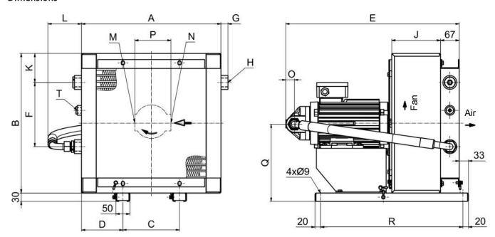
T Connection  $G \frac{1}{2}$  for temperature switch
