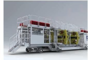
A remarkable feat of engineering – the Crossrail drilling rig, comprising two machine components, moves through the tunnels drilling more than 250,000 holes in the tunnel lining.
